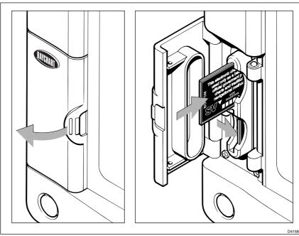
Figure 3-1: Removing the Chart Card
